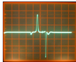
Typical Output Vertical 100mV/div Horizontal 20ms/div
