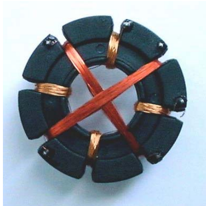
Fig 1 A typical ring fluxgate magnetometer showing the two sense windings and the toroidal excitation winding.
